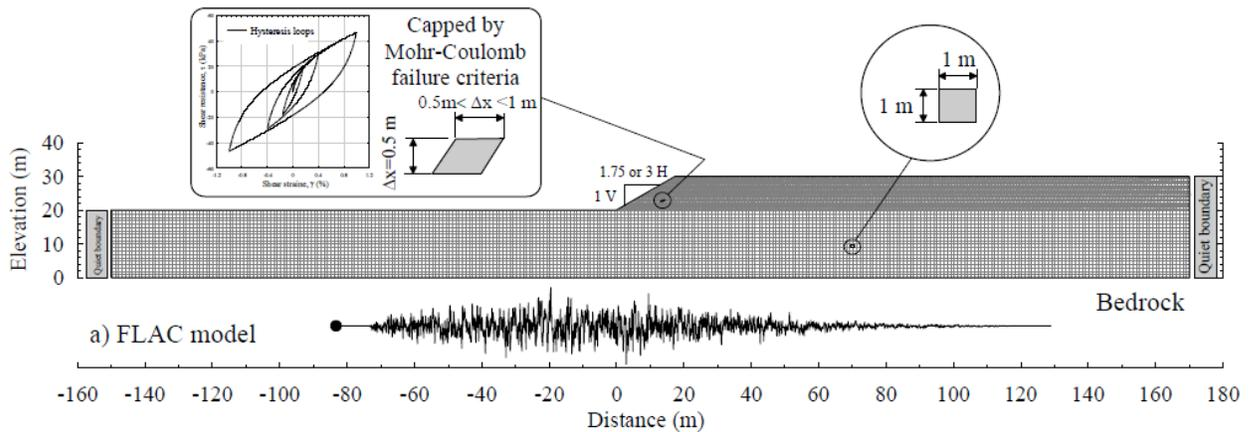
Figure 2: Basic characteristics of the slope, meshing, and associated boundary conditions. Model shown for geometry of  $H_S=10$  m and deposit height of  $H_D=20$  m. (Karray et al. 2018a).
