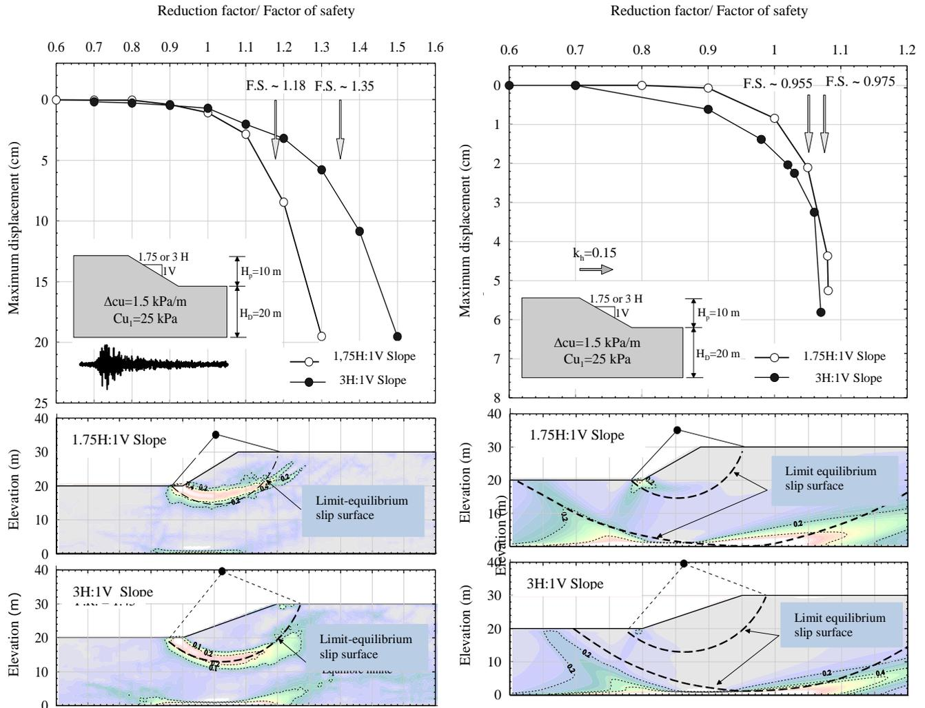
Figure 1: Comparison between dynamic analysis and failure surface obtained using a constant seismic coefficient  $kh=0,15$  proposed by NBCC (National Building Code of Canada) for seismic zone 4. Adapted from Karray et al. (2017c).
