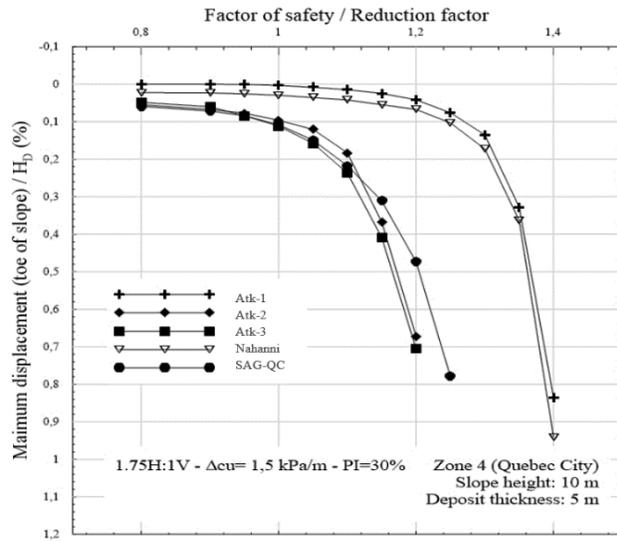
Figure 5: Relative displacement factor of safety curve for 1.75H:1V,  $H_s= 10$  m and  $H_D= 5$  m. The factor of safety varies between 1.32 and 1.14.
