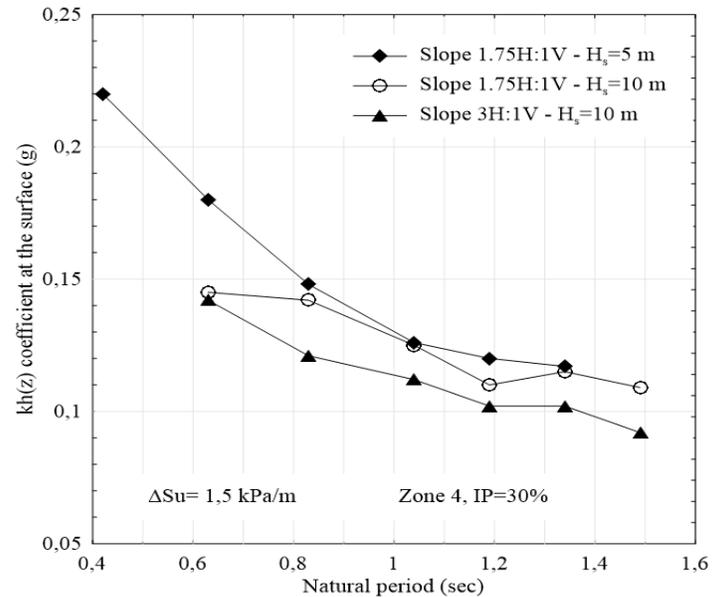
Figure 6: Proposed seismic coefficient as a function of natural period, with consideration of different earthquakes compatible with seismicity of Eastern Canada. Results shown for seismic zone 4, plasticity index of 30% and 1.5kPa\m shear strength profile.
