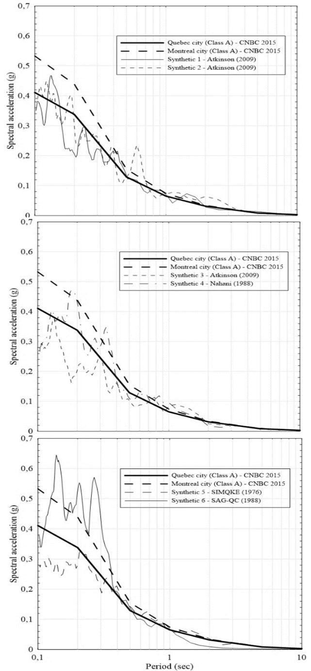
Figure 4: Acceleration spectra for earthquakes spectrums compatible with Quebec seismic zone 4 used in this study determine the factor of safety corresponding to 0.2% of the maximum displacement, corresponding to plastification of the slope. Moreover, the development of the slip surface is examined throughout the same shear strength reduction analysis. However, the pertaining results are not presented here because the space limitation.
