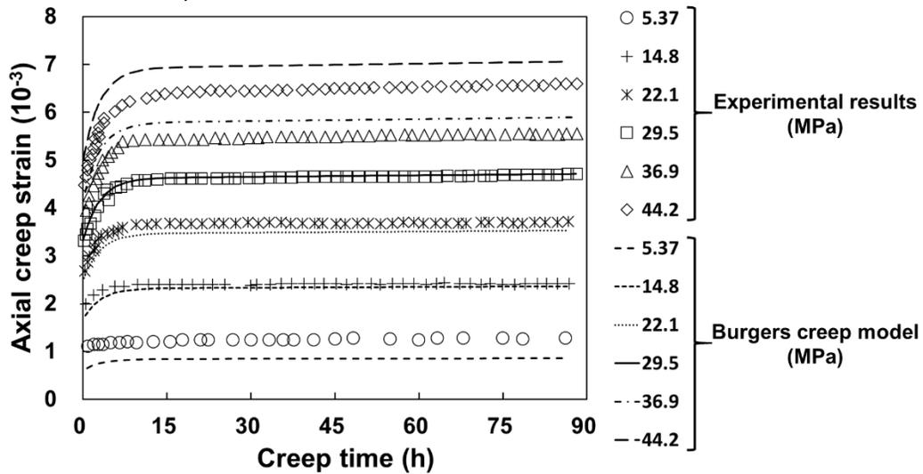
Figure 4. Strain evolutions measured with a cylindrical rock submitted to a confining stress of 6 MPa at different deviatoric stress levels (experimental data taken from Zhao et al. 2017); on the figure are plotted one description and five predictions of the experimental results using the Burger creep model with the model parameters shown in Table 3.
