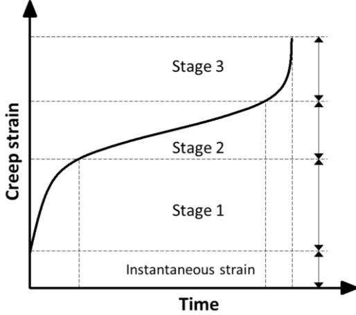
Figure 1. A schematic presentation of creep behavior of rock (after Farmer 2012).
