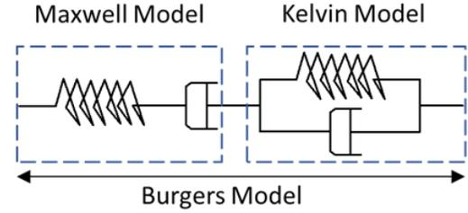
Figure 2. Schematic illustration of the Burgers creep model composed of Maxwell model and Kelvin-Voigt model (after Goodman 1989).
