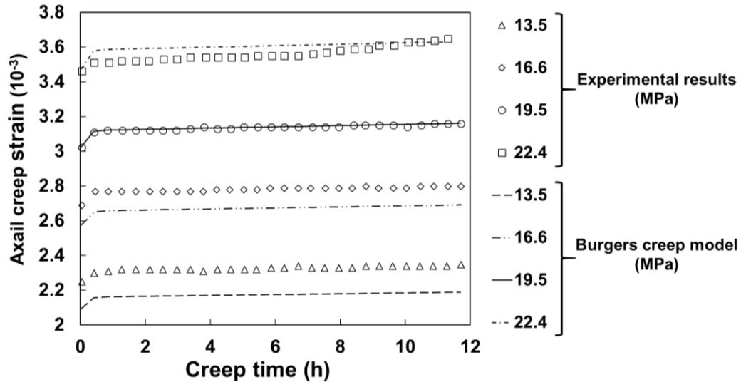
Figure 3. Application of the Burgers creep model for one description and three predictions of the strain evolutions of a cylinder rock, submitted under different constant axial stresses (experimental data taken from Wang et al. 2017); Burgers creep model parameters are given in Table 1.
