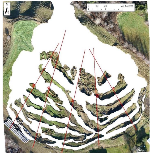
Figure 7. Delimitation of the grabens and the location of the 5 cross sections
