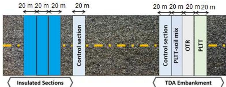
Figure 2. Schematic plan of the IRRF test road
