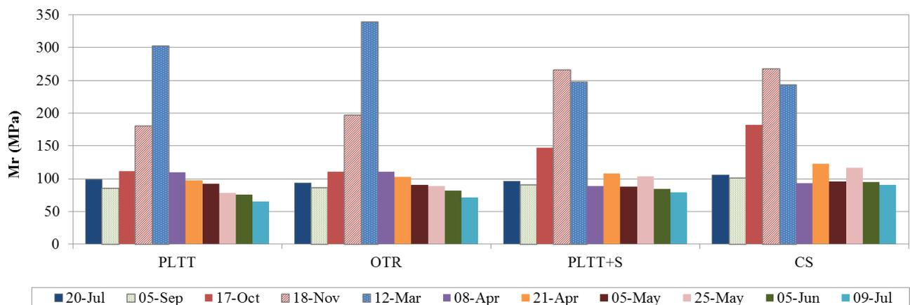
Figure 7. Resilient modulus of different sections
