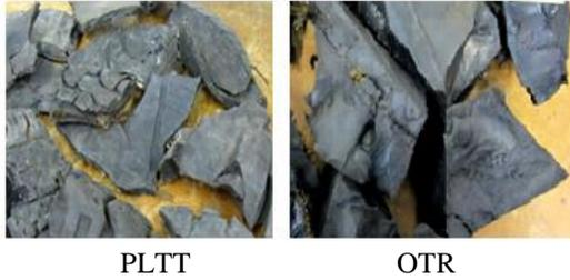
Figure 1. Tire-derived aggregate material
