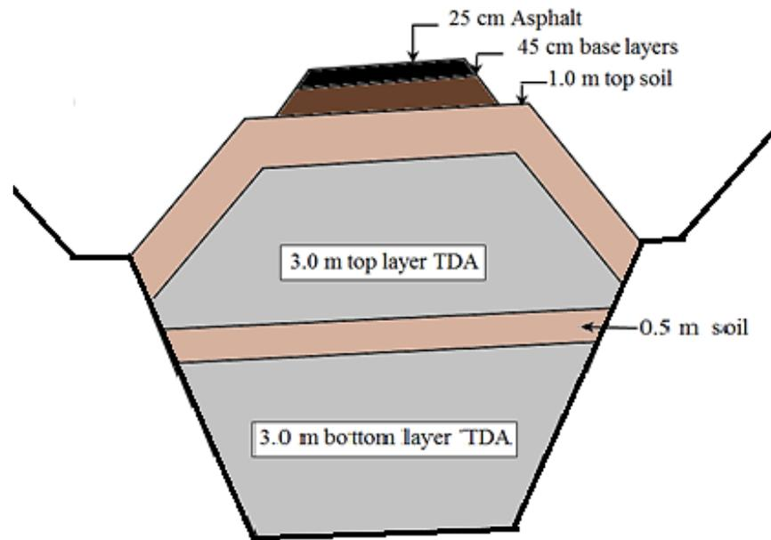
Figure 3. Typical pavement section including tire embankment
