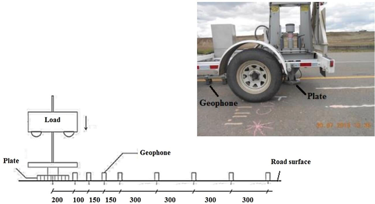
Figure 4. FWD device and geophones configuration
