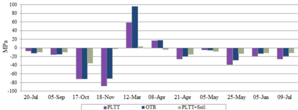
Figure 8. The difference in resilient modulus between the tire sections and the control section.
