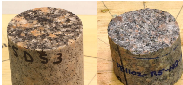
Figure 3. NQ3 (45 mm) Pointe Du Bois core: (left) saw cut specimen, and (right) fracture specimen
