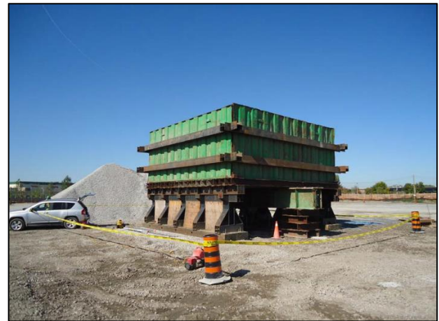
Figure 11. Photo of Foundation Load Test frame.
