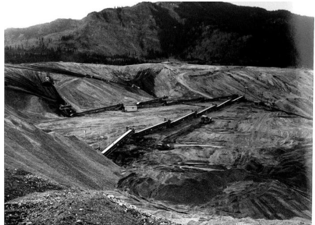
Figure 3 South Moraine – collector conveyors
