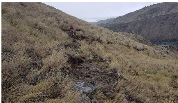
Figure 6. Two additional boreholes for matric suction monitoring. BH 18-1 (top) and BH 18-2 (bottom)
