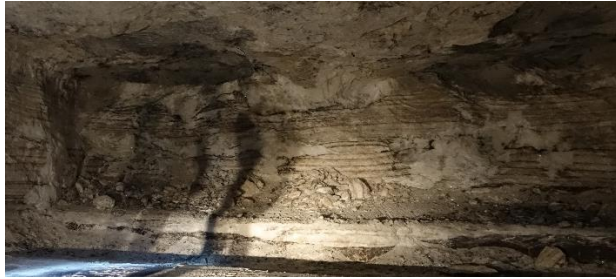
Figure 4: Active working face at Ojibway. Rock salt and anhydrite strata are present across the face and are discernable by coloration.
