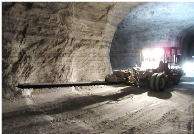
Figure 2: Electric undercutter used at the Ojibway mine to create an undercut kerf at the base of the face. Undercutter bar is 4 meters long and creates a 37 cm thick kerf.
