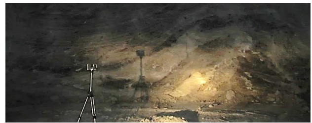
Figure 6: A series of folds at the Pugwash mine along a mined out drift. Deformed rock salt layers of different purity are intertwined with dark folded bands of massive anhydrite.
