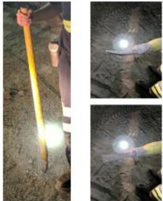
Figure 3.1: Pictures of a scaling bar, typically used to perform secondary scaling and sound surfaces for voids.
