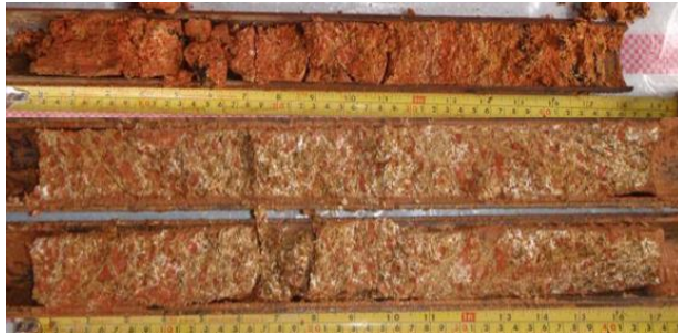
Figure 2. Typical photograph of saprolite soil
