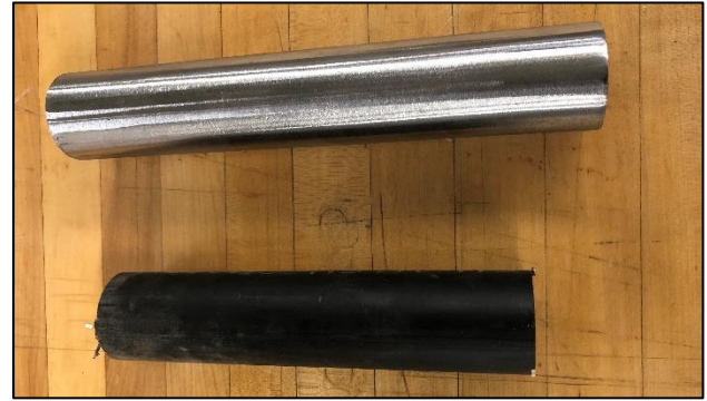
Figure 7. Top – After the corrosion protection coating has been removed. Bottom – Prior to sample preparation.
