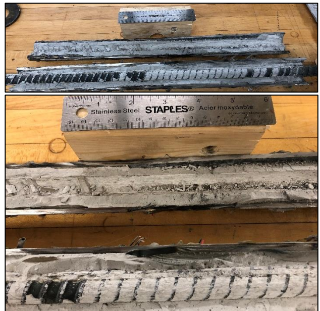
Figure 20. Top. 500 mm sample cut diametrically. Bottom - Center of 500 mm sample illustrating grout shearing.
