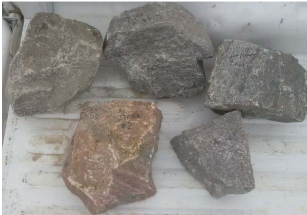
Figure 3. Samples collected at the site for coring and UCS testing on select samples.
