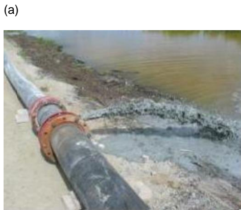
Figure 2. (a) Hydraulic deposition of Goldex mine tailings at the Manitou site (from Pabst 2011); (b) particle sorting in conventional tailings deposition (from Blight 2009)
