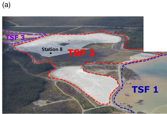
Figure 1. (a) The three tailings storage facilities (TSF 1, TSF 2 and TSF 3) at the Manitou site and location of Station 8 in the TSF 2 (adapted from Éthier 2018); (b) A schematic representation of a monolayer cover with an elevated water table (adapted from Ouangrawa et al. 2010)
