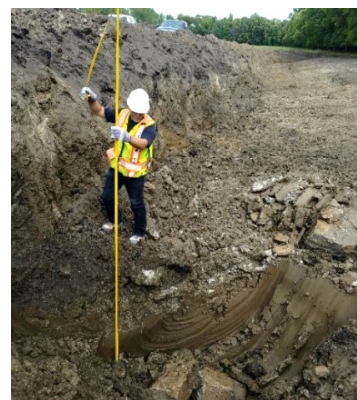
Figure 3. Block sampling at site 1
