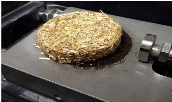
Figure 4. Material condition after direct shear test.
