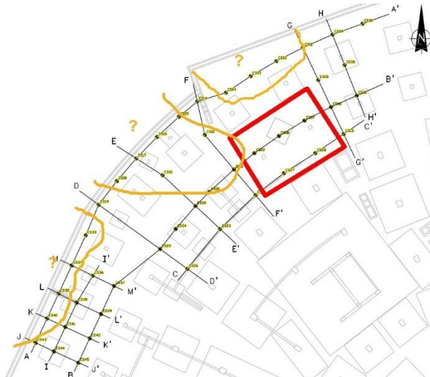
Figure 11. Excavation boreholes and cohesionless soil
