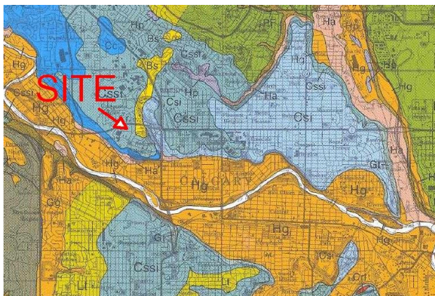
Figure 2. Site location within lacustrine sediments (blue)
