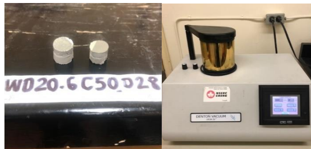
Figure 1: Photographs of two gold-coated samples (L) and gold laboratory Vacuum Thin film Thermal evaporator (R).
