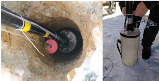
Figure 4. Downhole survey with GPR unit protected
