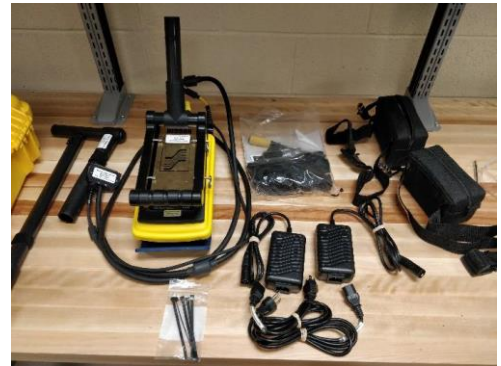
Figure 3. 1GHz Noggin GPR unit
