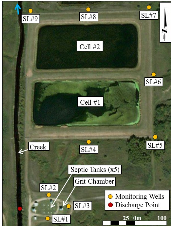
Figure 3. Site layout. The nomenclature SL# is used to identify the monitoring wells located near the WWT lagoon (Imagery Microsoft Corporation 2018).
