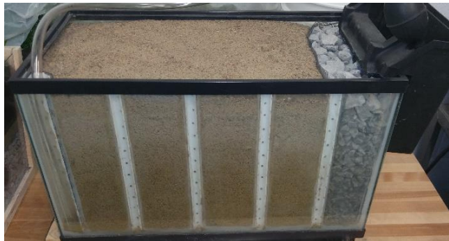
Figure 8. Pump test demonstration model
