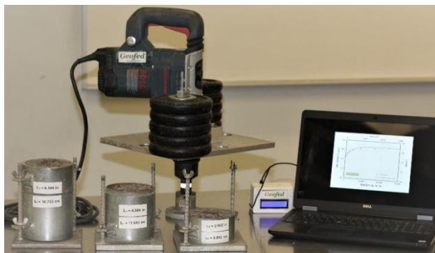
Figure 6. Batch testing with vibratory compactor
