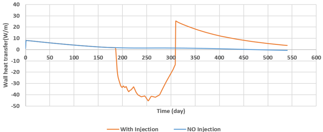
Figure 12. Average heat transfer per length for middle pipe with and without injection of water as heat source.
