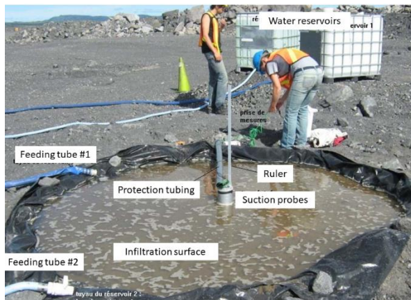
Figure 3. Photo of one of the infiltration ponds used for the infiltration tests (Lessard 2011).
