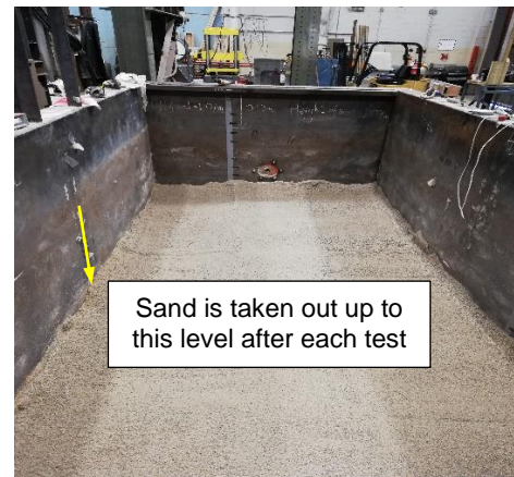
Figure 3. Bedding for MDPE pipe in loose sand inside the testing cell
