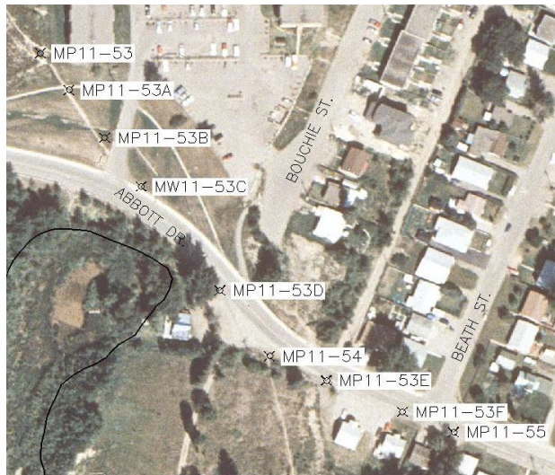
Figure 9. Additional survey hub installed along Abbott Drive (the West Quesnel slide) to improve the accuracy of the differential displacement measurements.
