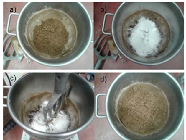
Figure 4. Preparation of lime-amended SaSM: a) SaSM without lime, b) adding lime to SaSM, c) mixing of the lime-amended SaSM, d) homogeneous lime-amended SaSM at the end of mixing
