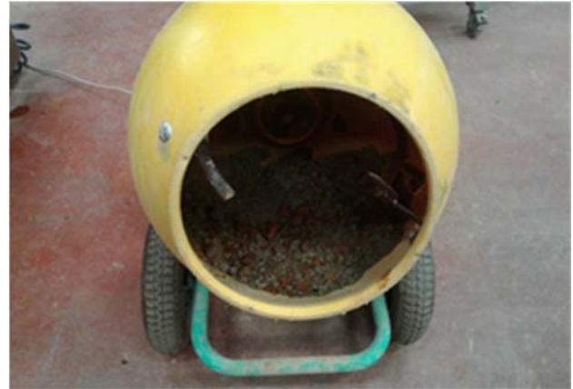
Figure 3. Mixer used for the preparation of SaSMs
