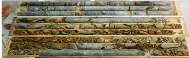
Figure 2. Anorthosite and shear zone, Mine Campbell (BH16-MC-C5A, 0 to 25.2 m)
