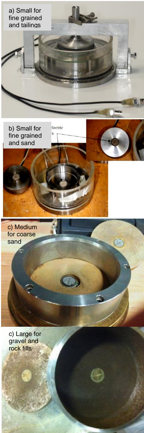
Figure 7. Piezoelectric sensors installed in four different odometer cells to measure shear wave velocity fine grained soils or tailings (a) to sand (b,c) and Rock fills (d).
