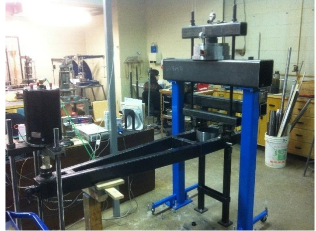
Figure 10. Experimental setup for testing Rock fills samples.
