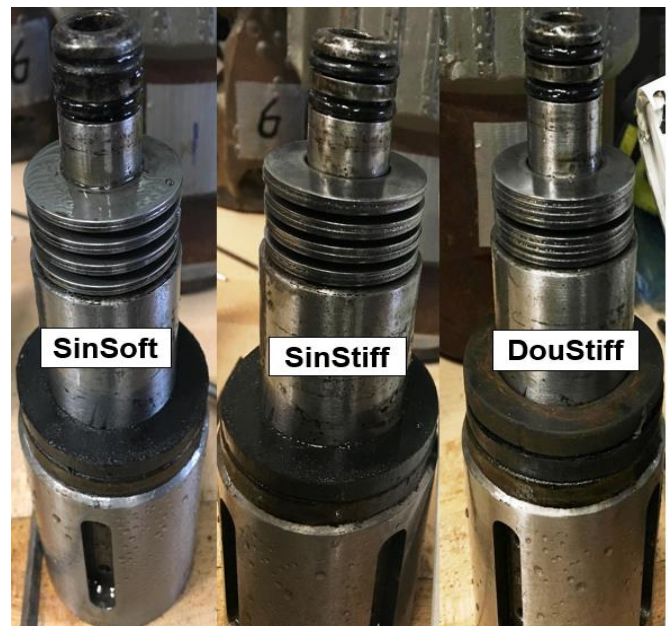
Figure 2. Configurations of the Belleville spring setting in the p-VARD tool, with 8 sets of single parallel soft springs (left), 8 sets of single parallel stiffer springs (middle) and 4 sets of double parallel stiffer springs (right).
