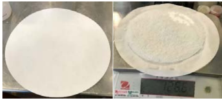
Figure 3. Initial filter paper and hydrogel SAP after filtration
