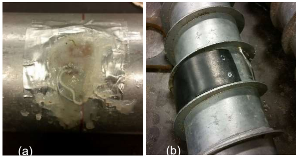
Figure 4. Strain gauge protection a) epoxy and aluminum foil, b) steel sheet casing
