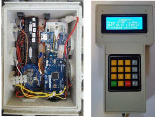
Figure 3. Data Acquisition System (DAQ) system (left) and the remote control for the driller (right)
