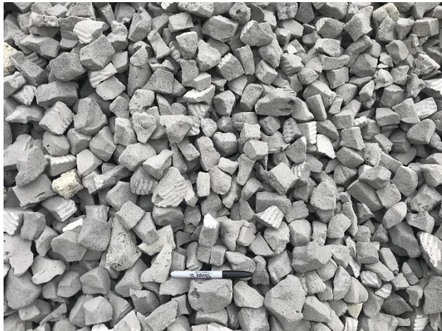
Figure 2. Foamed glass aggregate manufactured by AeroAggregates of North America. Note the permanent marker in the photo for scale.
