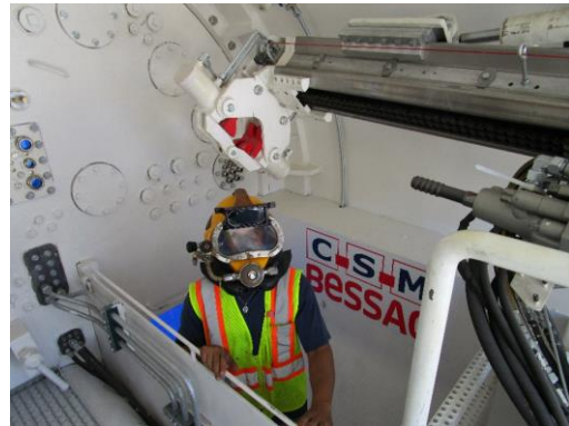
Figure 5. Diver pit for cutter change in the wet
