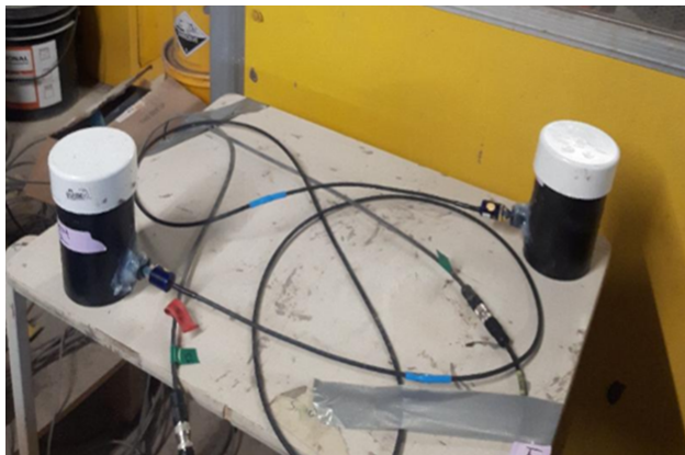
Figure 2. Two T5x tensiometers installed into two replicate columns.
