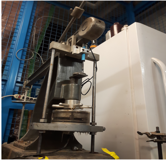
Figure 1. Modified oedometer with T5x tensiometers installed in the base and connected to DL 2e data logger.
