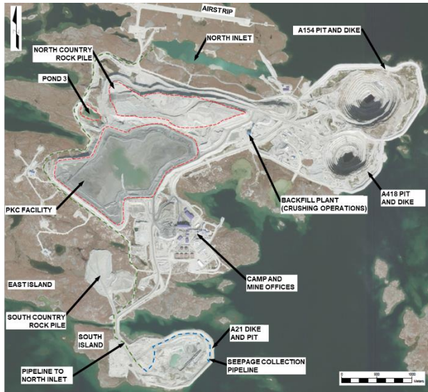
Figure 1. 2018 satellite image showing the Diavik Diamond Mine Site, and approximate locations of site infrastructure.
