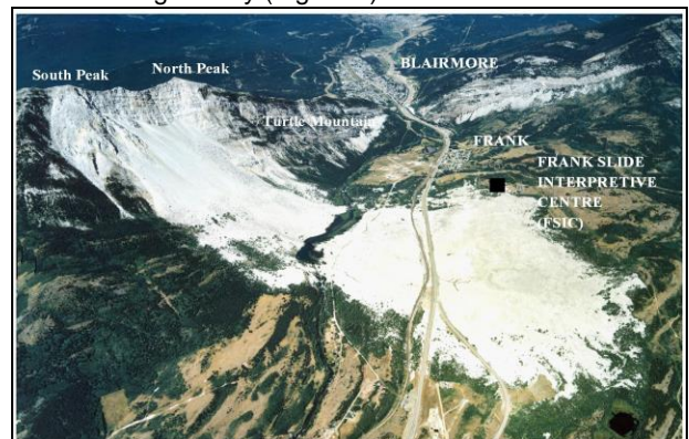
Figure 7. Photo of the Frank rock avalanche scar and deposit showing the north and south peaks at the top of Turtle Mountain. The road across the deposit is the Trans-Canada highway.
