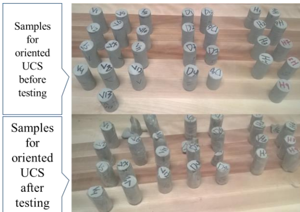
Figure 7. Sandstone core samples before (top) and after (bottom) OUCS testing
