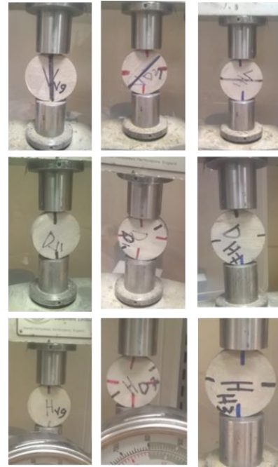
Figure 4. Procedure of OITS test on sandstone disk sample
