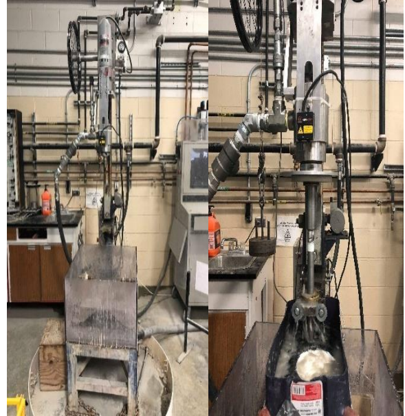
Figure 2. Small Drilling Simulator (left) and cutting collection system installed (right).
