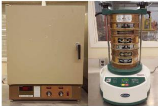
Figure 4. Oven and standard sieving machine used to sieve analysis.
