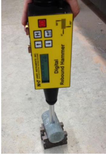
Figure 9. Hardness measurement by a rebound hammer
