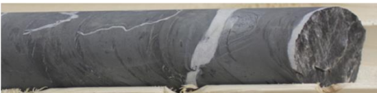
Figure 3. Drill core (NQ, 47.6 mm diameter) examples of rock units in this study from the Legacy skarn deposit
