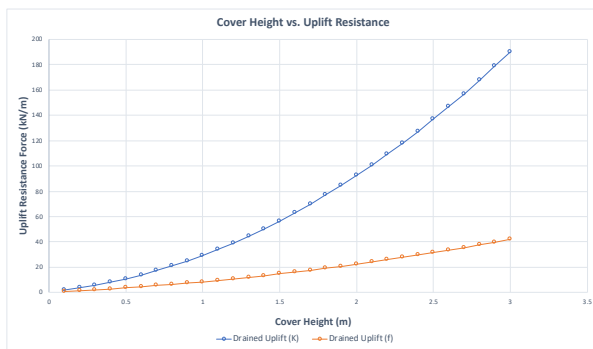
Figure 6: Drained Uplift Resistance vs. Cover Height
