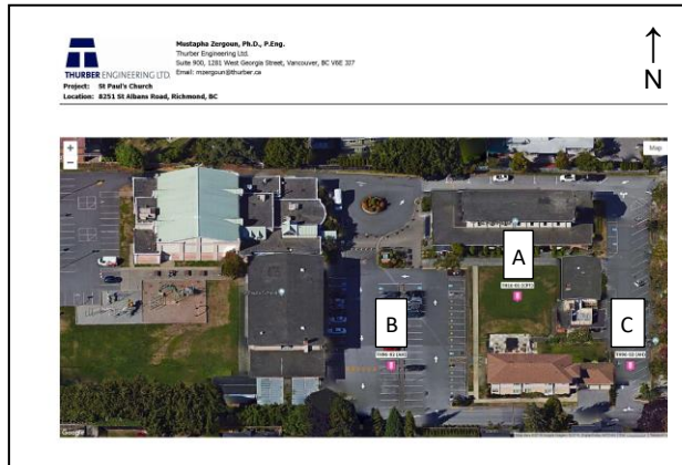
Figure 2 Test hole location plan in 2016 site investigation A = CPT96-01 B = AH96-01 C = AH96-02
