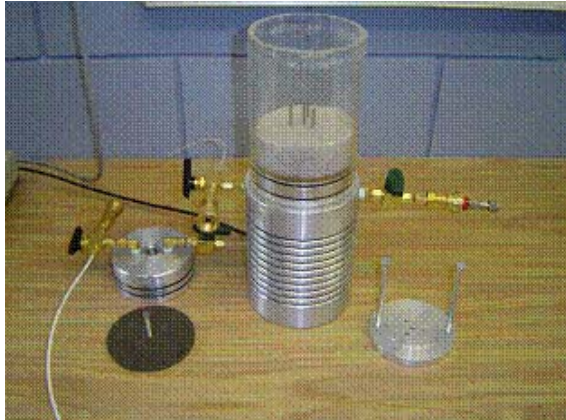
Figure 3. Specimen Preparation after the first layer is complete
