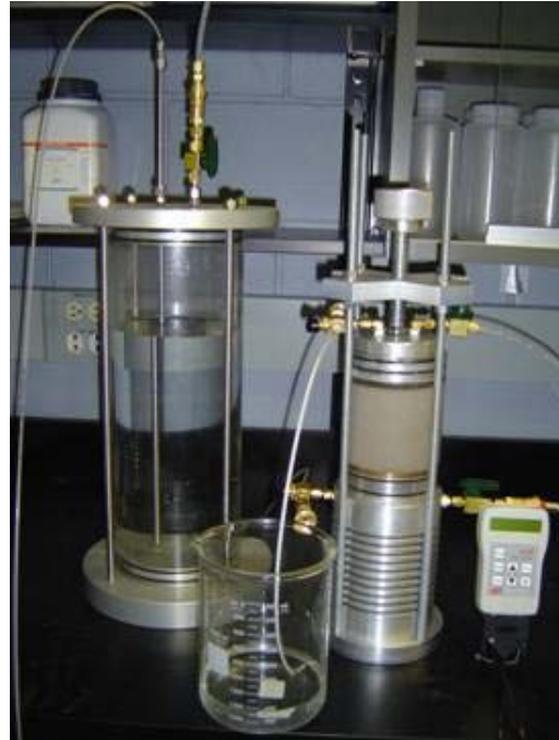
Figure 4. Specimen CO 2 Cycling and Saturation Procedure
