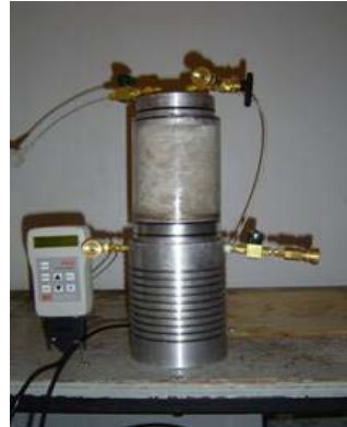
Figure 5. R-11 Hydrate Specimen at Test Completion
