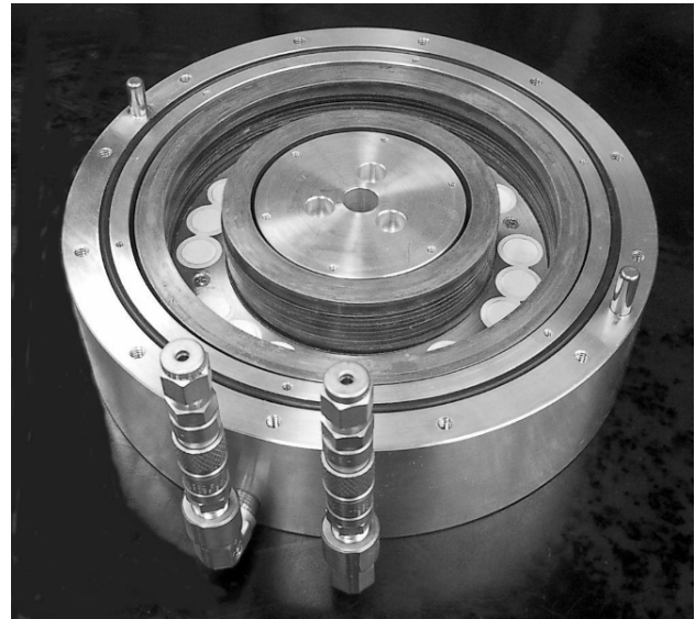
Figure 6 Base of unsaturated ring shear cell with ceramic disks and inner confining ring stacks in place.
