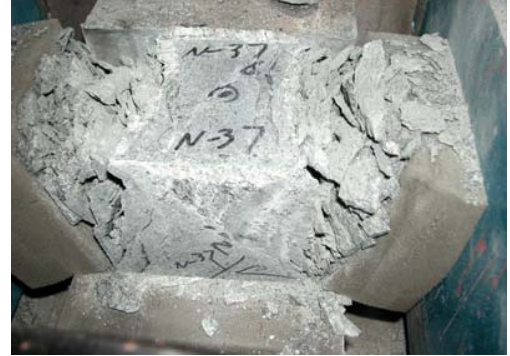
Figure 10. Top and side views, failure mode, 169.9 MPa confinement test, 0.75 MPa/sec loading rate
