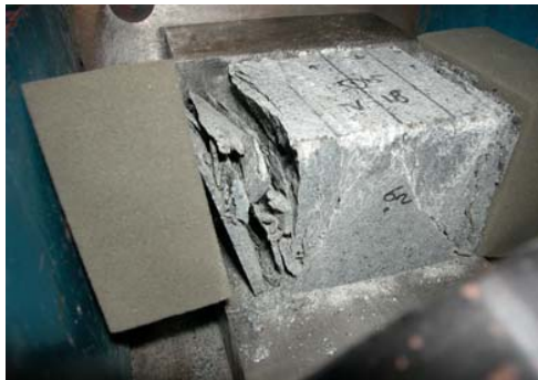
Figure 12. Top and side views, failure mode, 101.6 MPa confinement test, 2.25 MPa/sec loading rate.
