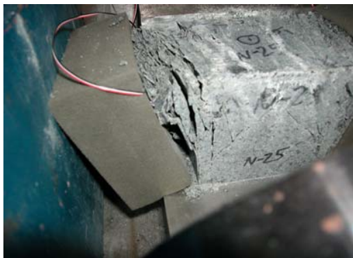
Figure 9. Top and side views, failure mode, 150.6 MPa confinement test, 0.75 MPa/sec loading rate.
