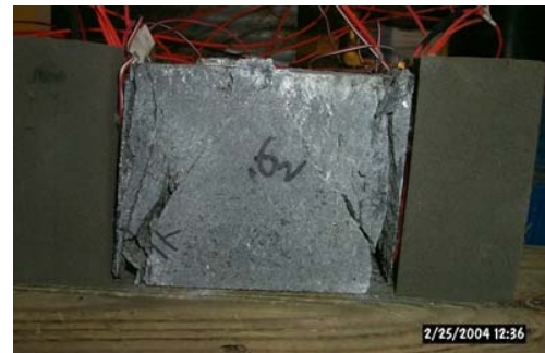
Figure 14. Top and side views, failure mode, 170.5 MPa confinement test, 2.25 MPa/sec loading rate.
