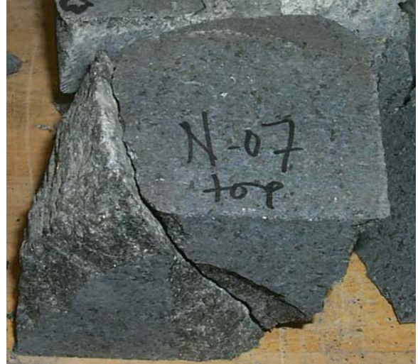
Figure 6. Failure mode, uniaxial test, 0.75 MPa/sec loading rate.
