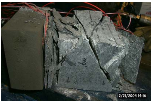
Figure 13. Top and side views, failure mode, 150.7 MPa confinement test, 2.25 MPa/sec loading rate.
