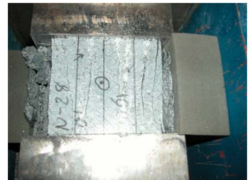
Figure 10. Top and side views, failure mode, 169.9 MPa confinement test, 0.75 MPa/sec loading rate
