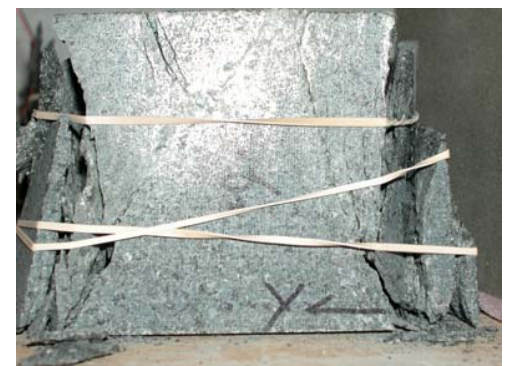
Figure 11. Top and side views, failure mode, 51.3 MPa confinement test, 2.25 MPa/sec loading rate.
