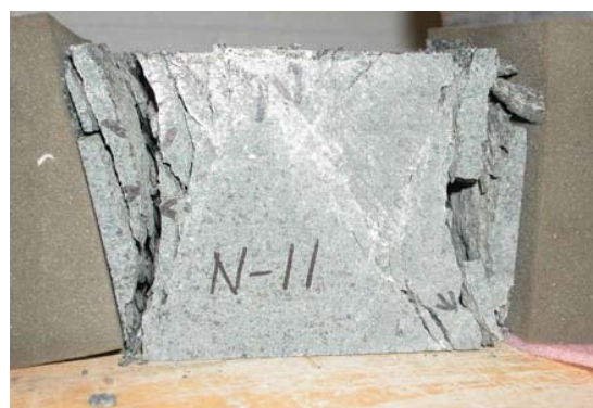
Figure 7. Top and side views, failure mode, 52.3 MPa confinement test, 0.75 MPa/sec loading rate.
