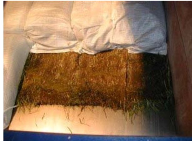
Figure 10. Photograph of sandbags / sod following testing in large-scale (1m² plan view) direct shear box
