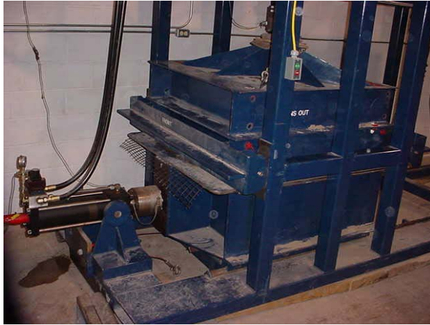
Figure 3. Photograph of large-scale direct shear apparatus (1m 2 plan area)
