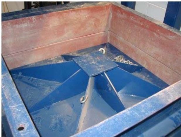
Figure 4. Photograph of normal load platen for large-scale apparatus
