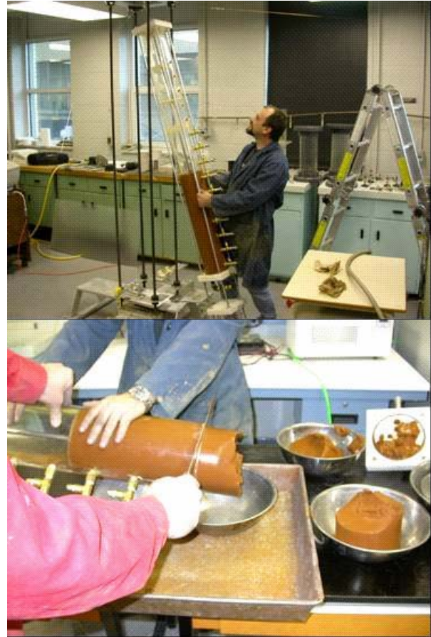
Figure 4. Pictures of the dismantling of the column and sampling of the sludge
