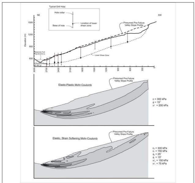
Figure 5. Typical cross section of Downie Slide (top) showing location of shear zone (after Imrie et al., 1991). Output from finite difference models using the elasto-plastic M-C (middle) and elastic, strain softening M-C (bottom) constitutive relations. Contours represent shear strain increments at intervals of 1x10<sup>-1</sup>.
