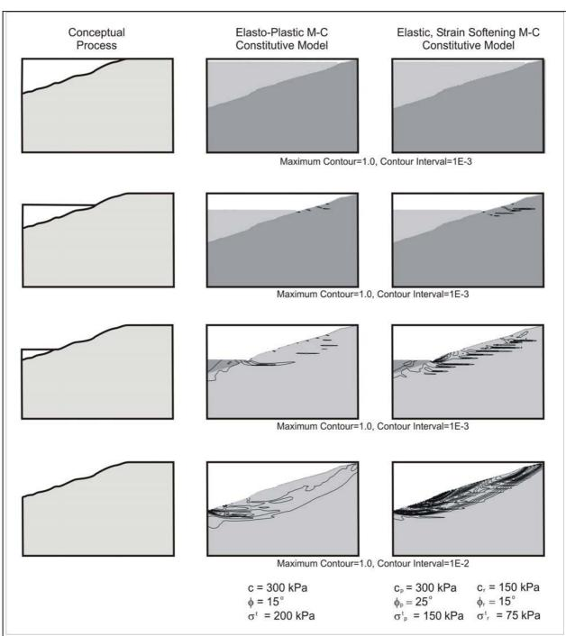
Figure 6. Comparison of shear strain increments for the finite difference model at different stages of deglaciation using elasto-plastic M-C and elastic, strain softening M-C constitutive relations. Note varying contour scales and the increased grid dependency for early shear propogation in the elastic, strain softening constitutive model.
