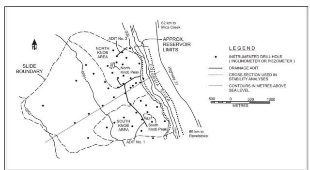
Figure 1. Plan of Downie Slide, showing the location of instrumented drill holes, drainage adits, north and south knobs, and the alignment of the cross section used in the numerical analysis (after Imrie et al, 1991).
