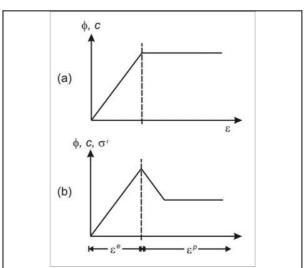
Figure 4. Schematics showing relationship between strain and material properties for (a) elasto-plastic M-C and (b) elastic, strain softening M-C constitutive laws.
